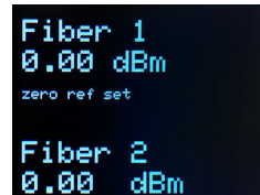
Display when RX unit is calibrated and connected to TX unit.
