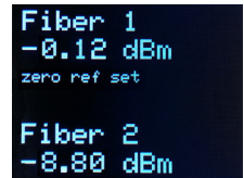
Example display of high attenuation in Fiber 2.
