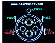
Example of display when there is an electrical short between conductors.
