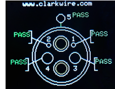
Display when there are no electrical faults present.
