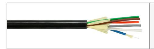
Heavy Duty Tactical Construction Individual Fiber Jackets Single-Mode or Multi-Mode Aramid Strength Member Polyurethane Jacket 2, 4, 6, 8 or 12 Fiber Elements
